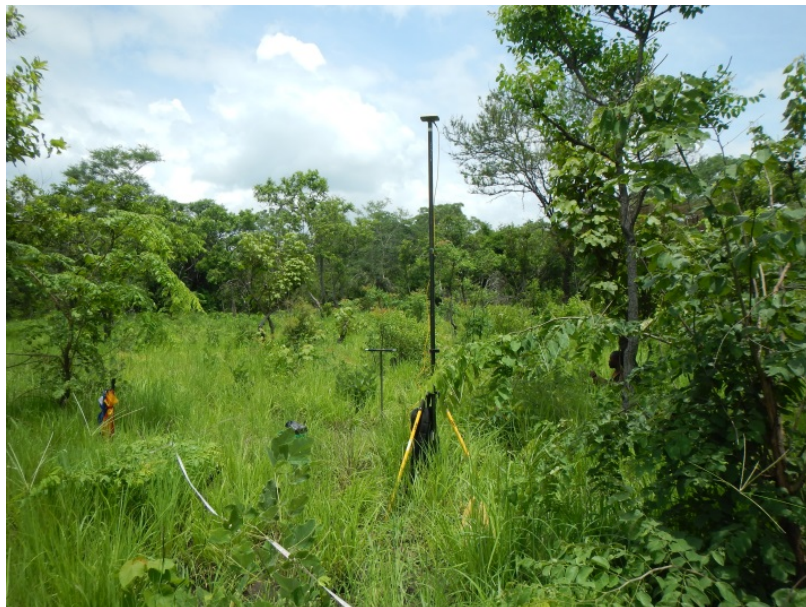
Fig. 2. Example of accurate GPS-recording of plot position for a circular NAFORMA plot. The coordinates of the center-point are determined. A 2.9 m tall antenna is used to improve reception of signals from the GPS satellites. Photo: Amiri Mahenge.
